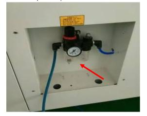
c) 3, put the whole bucket of flux into the bucket of the machine , and then put the infusion tube into the flux bucket, automatically extract liquid flux after start the machine.
